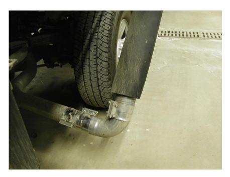
Consider 90° elbow at tail pipe to turn exhaust immediately (available from PatchBox or most exhaust shops)
