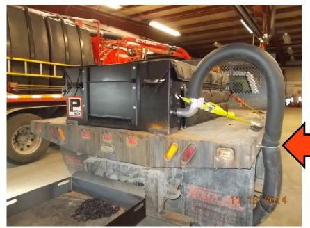
Consider sleeve to guide flex tube (2" thickness preferred to distribute load)
